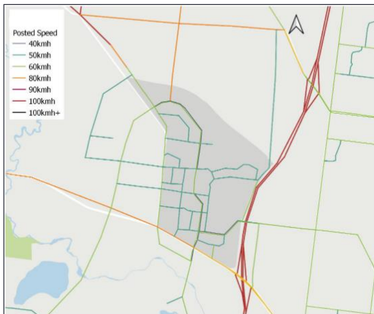
Figure 2: Future forecast road traffic speeds (source: reference (1))
