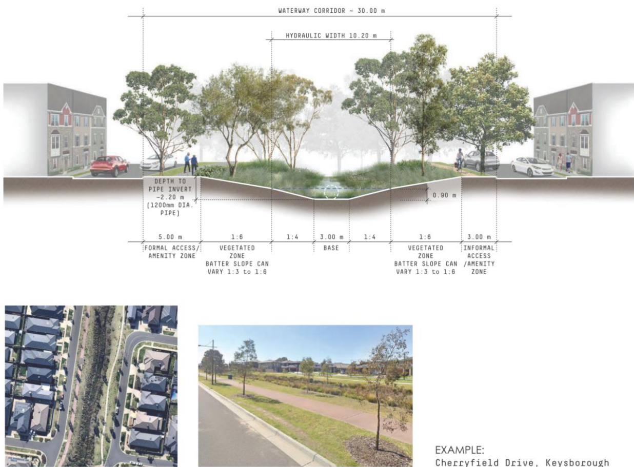
Figure 33. Schematic of a potential small hydraulic width waterway typology – a vegetated swale and example images
