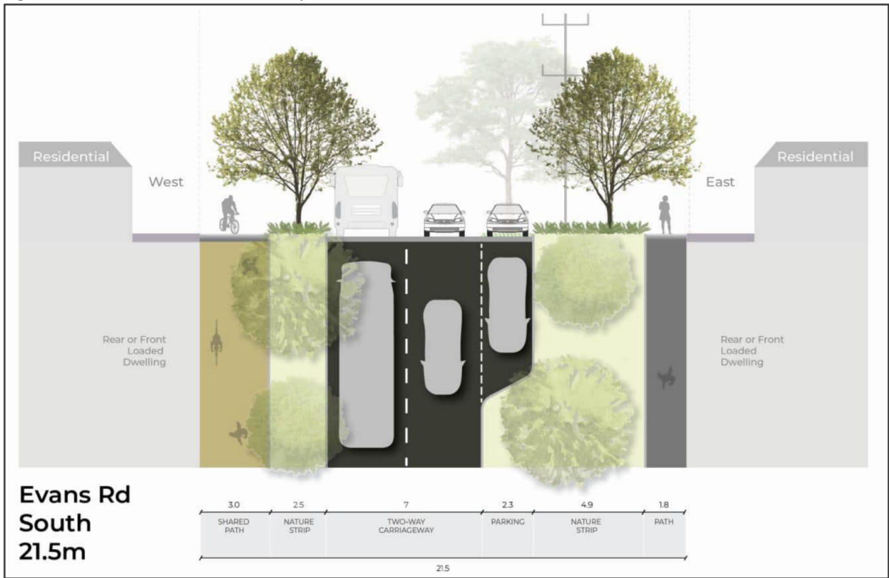
Figure 3-9: Evans Road – Councils FUS (adopted August 2024) Cross Section
