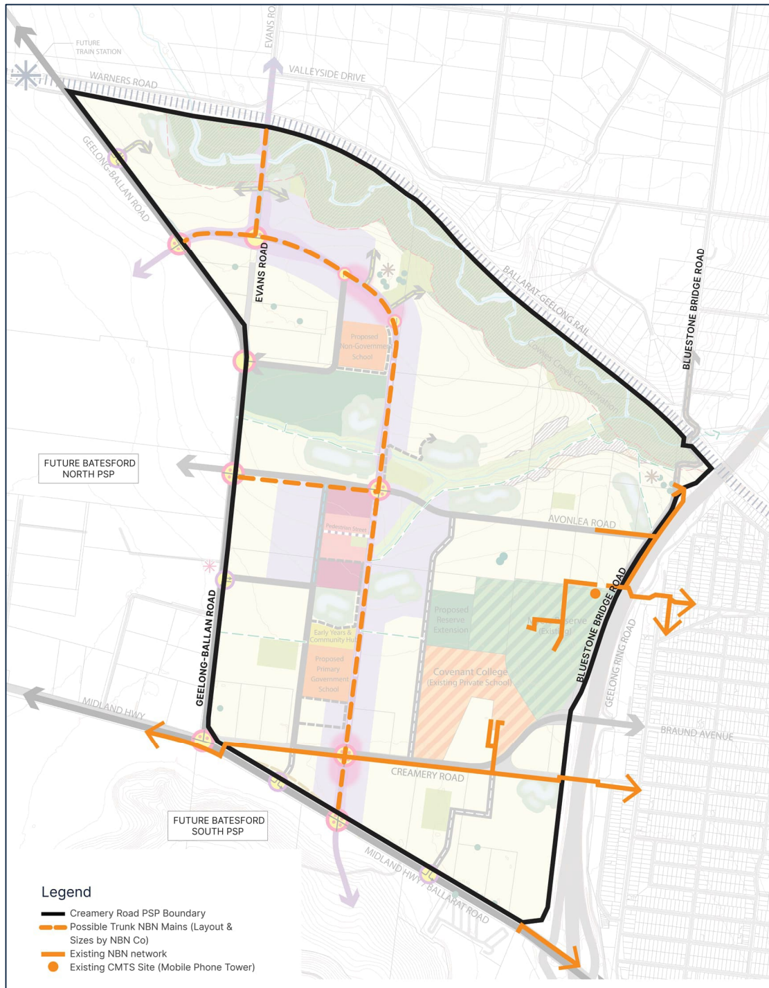
Figure 17: Existing and Proposed Communications Trunk Services
