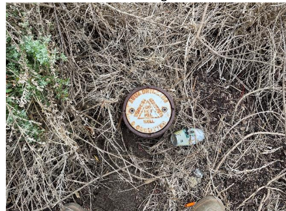
Photo 6: Groundwater monitoring well located onsite.
