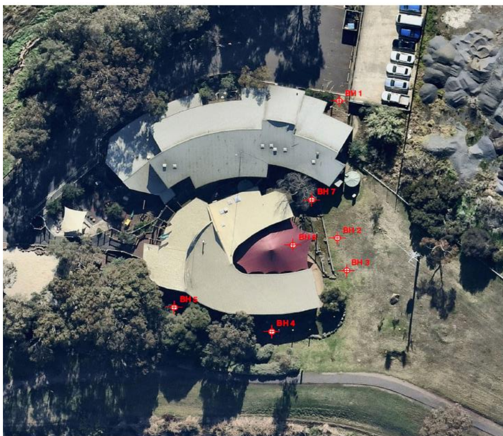
Figure 4 Bore holes for the 2021 geotechnical investigations (St. Quentin Geotechnical and Environmental Engineering, 2021).
